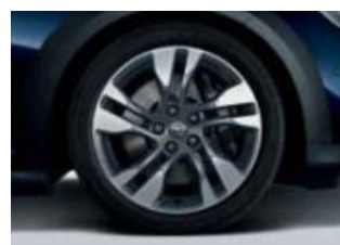
RV1: 18" alloy wheel, 8 J x 18, 5-twin-spoke design, bi-colour Technical Grey.
