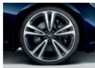
RTH: 20" alloy wheel, 8.5 J x 20, 5-double-spoke design, bi-colour Technical Grey.
