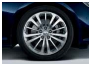
RCV: 18" alloy wheel, 8.5 J x 18, multi-spoke design, Bright Silver.
