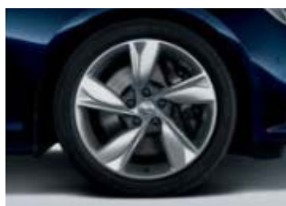
RCV: 18" alloy wheel, 8.5 J x 18, 5-single-spoke design, Bright Silver.
